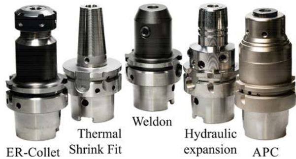
Fig. 1 Examples of the investigated tool holder systems
